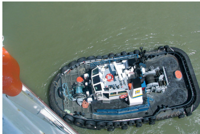
Following pilot Capt. John Armstrong's instructions, the 52-foot, 3,000-horsepower Z-drive tug Westminster Pride guides the Virana away from Richmond's Fraser Wharves.
